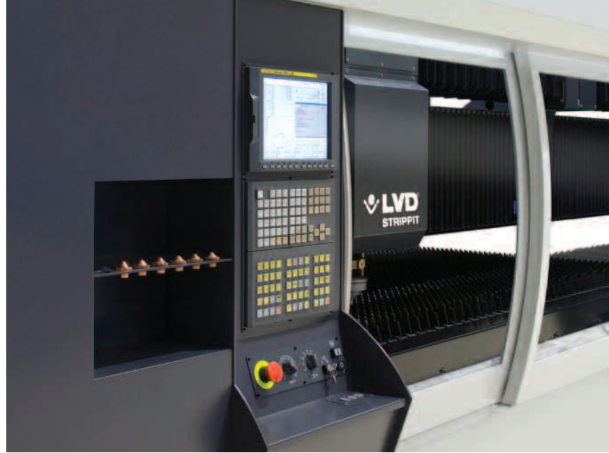
Integrated laser source and control
