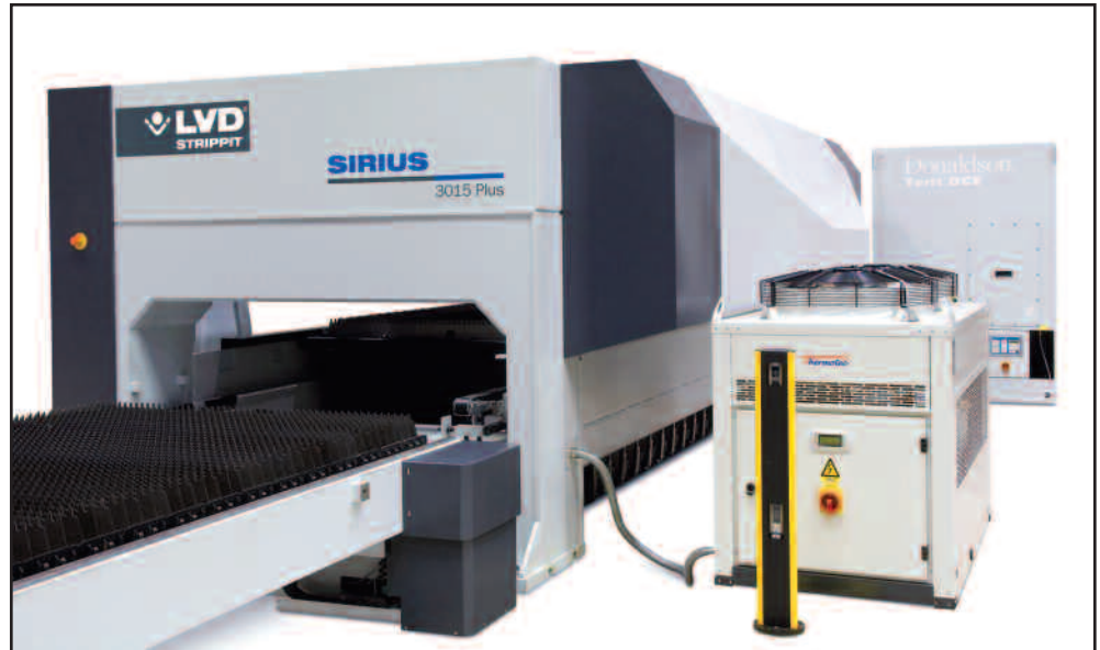
Sirius features an integrated exhaust system and cooling unit.
