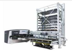
Automatic loading, unloading and storage of raw materials and finished parts.
