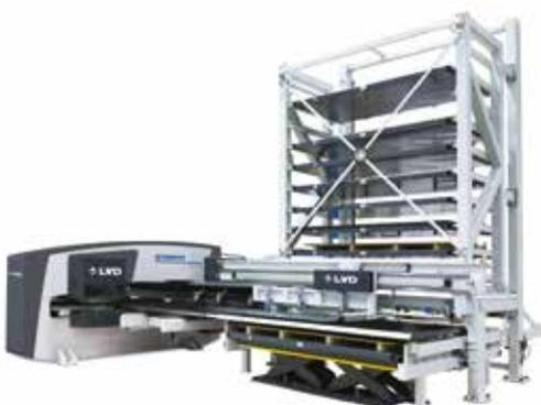
Automatic loading, unloading and storage of raw materials and finished parts.
