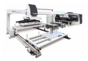
Advanced load/unload and part picking system with large stacking area.
