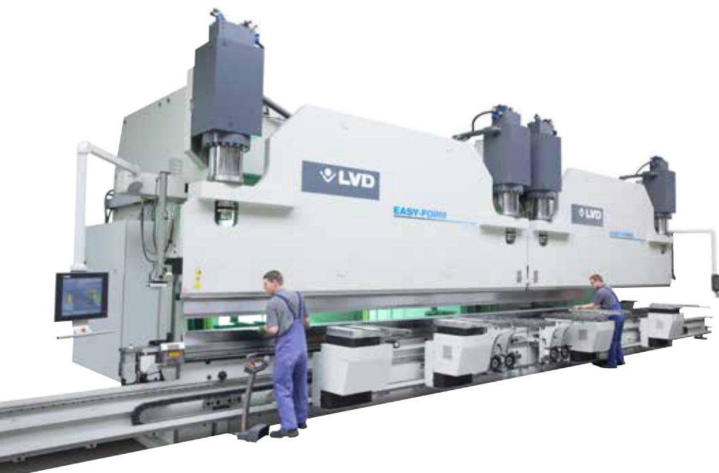
Tandem operation: Synchronized operation of two machines with a single master CNC control or independent operation of each machine with separate control, available with dissimilar tonnage and lengths in tandem configuration.
