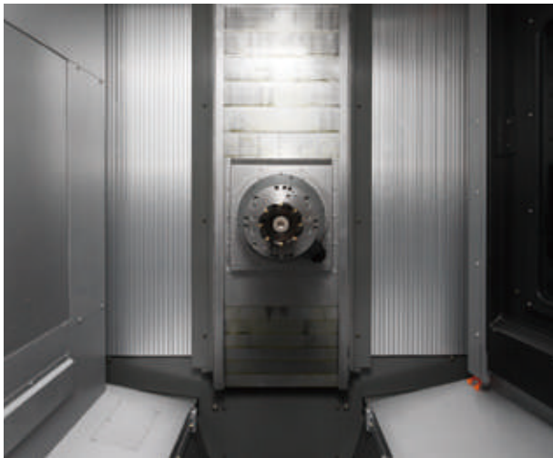
2 X-axis protective cover against chips To prevent damage to the cover from chip entanglement, an aluminum cover is adopted which operates jointly with the X axis stroke so that chips don't become caught.
