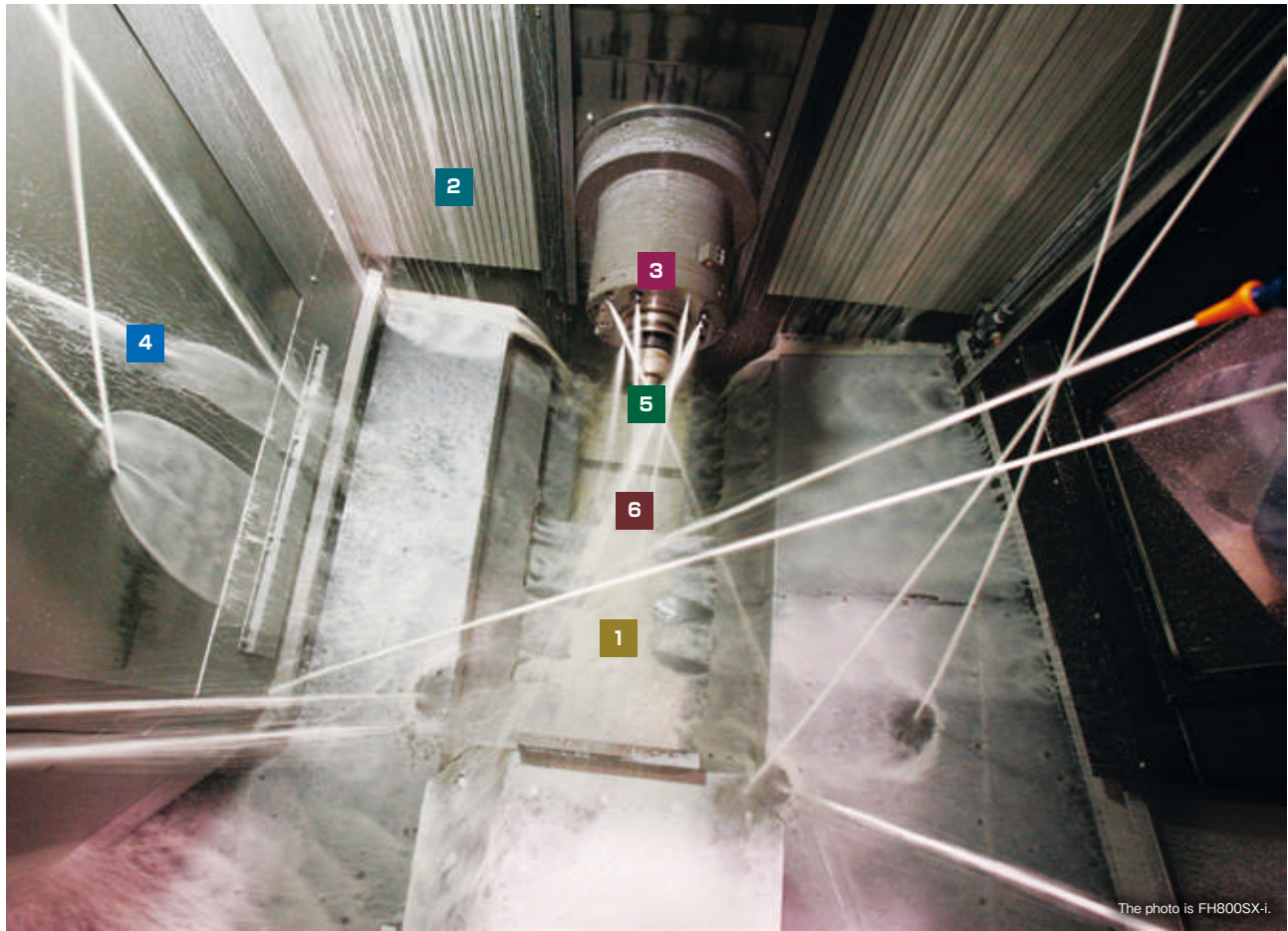
1 Center trough Smoothly processing machining chips with a large chip discharge port in the bed center.
