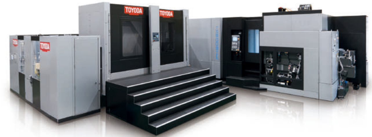
This is an example of FH800SX-I and RGV (rail guided vehicle)
