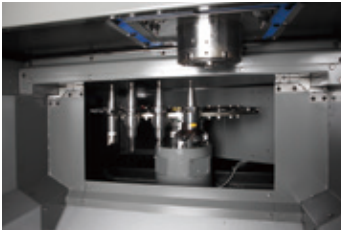
Direct magazine tool change method
