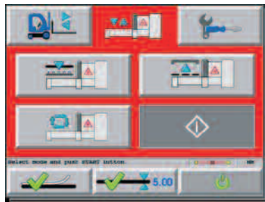
Control screens simplify programming of the automatic load/unload system
