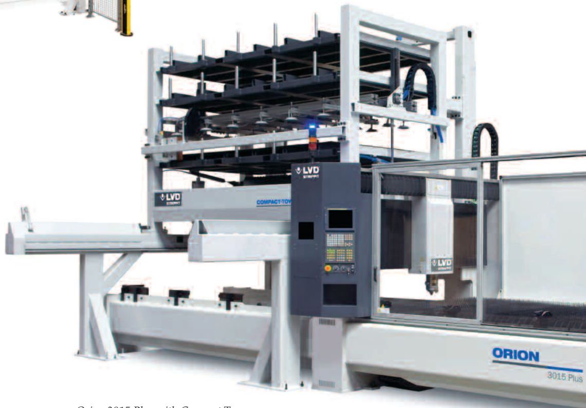
Automatic load/unload system
