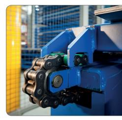
To remove the pallet from the bay, the draw hook engages in the driver.
