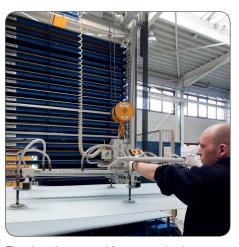
The sheet is removed for processing by means of a suction mechanism.
