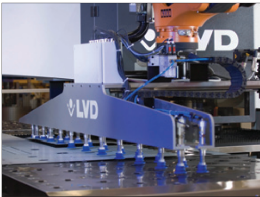
Pick-Sort system loads full size sheets and automatically retrieves and stacks individual punched parts.
