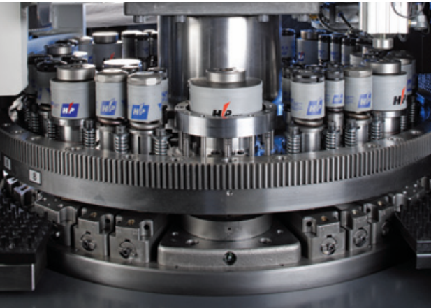
A large capacity turret features 48 stations.
