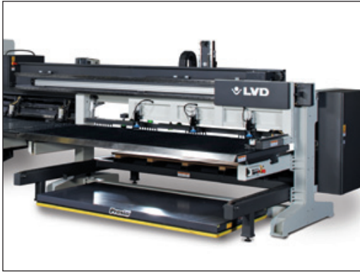
Load/unload system features full brush table for reduced part scratching.
