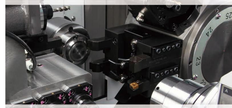
A sliding headstock type automatic lathe that encompasses the entire process Mounted Y-axis on three tool-posts, Turret, Gangtype tool post and Back tool post
