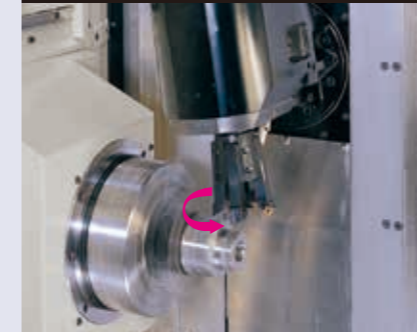
Multi turning holder to index in 4 positions
