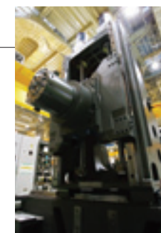
Y-axis dual ball screw drive, adopted in FH550SX, FH630SX and FH800SX
