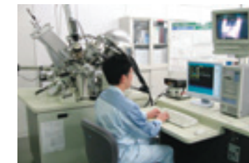
Using X-ray photoelectron spectroscopy to analysis fine matter adhered to a machined surface
