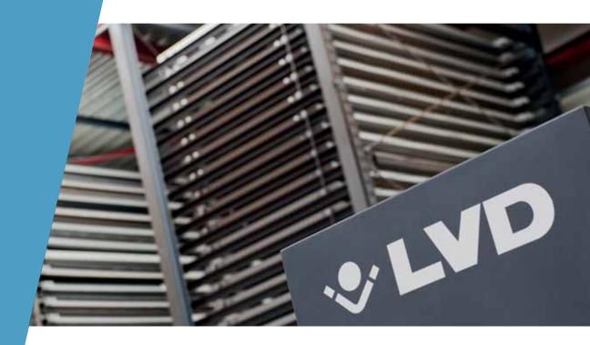
The MOVit Warehouse Automation System (WAS) provides the ultimate in automatic material storage and retrieval with a customizable number of tower storage units beginning with a minimum of four towers, in a single or double row configuration. WAS keeps sheets in continuous flow for uninterrupted production and full lights-out operation, and can be connected to multiple laser cutting machines in 3015 or 4020 formats.
