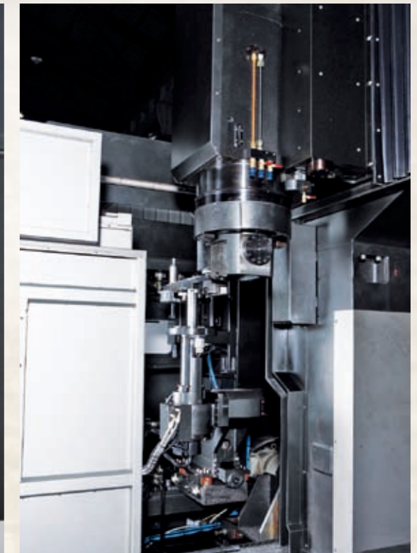
• Automatic tool exchange system in vertical/horizontal/ turning tool.
