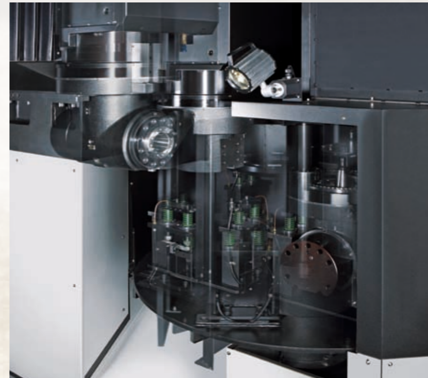
• Automatic head exchange system in vertical/horizontal/ turning head.
